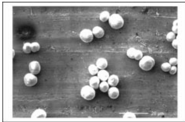
Figure 8. SEM micrographs of PCC 2 calcined at 400°C (pure calcite).
